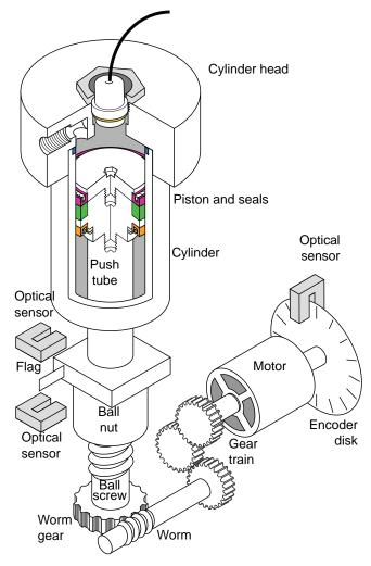
**Figure 1: Component identification**
