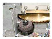
Figure 5: Lube wheel (Saturate with ALMASOL 609)
