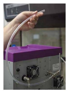
Figure 3: Filling the P-trap drain. Keep liquid level lower than the top of the system
