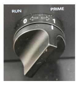
Figure 1: Turn the valve to the Prime position
