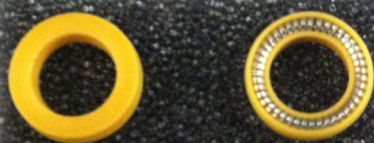
Figure 12, Example of polymer side vs. energizer side of seal. Note stainless steel energizer shown. Seal could have fluoropolymer o-ring energizer instead (black o-ring).
