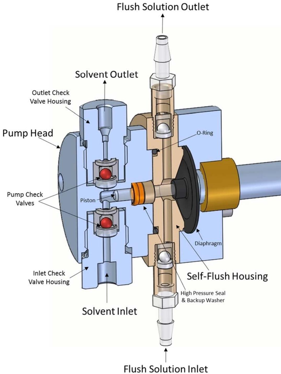
*Figure 1, MX-Class Self-Flushing Pump Head
