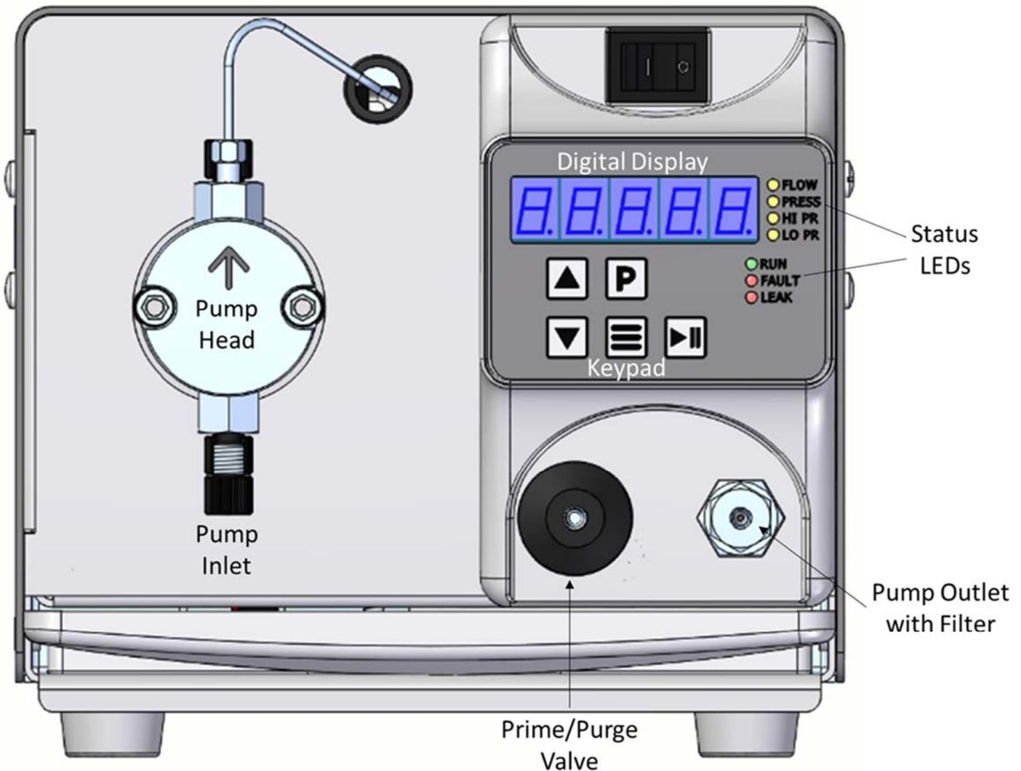
Figure 2, MX-Class Pump Front Panel Components
