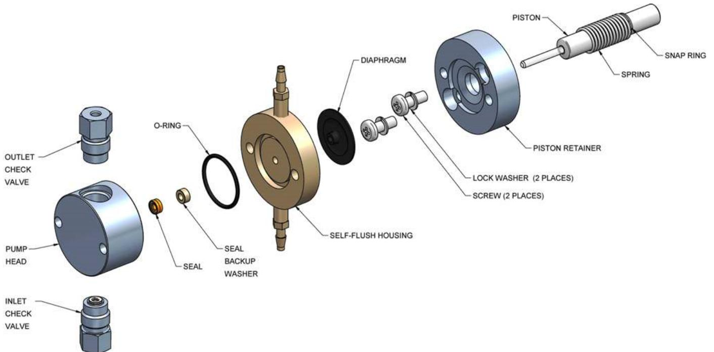
Figure 7, Stainless Steel Self-Flushing Pump Head Assembly
