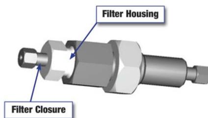
Figure 5, Outlet Filter
