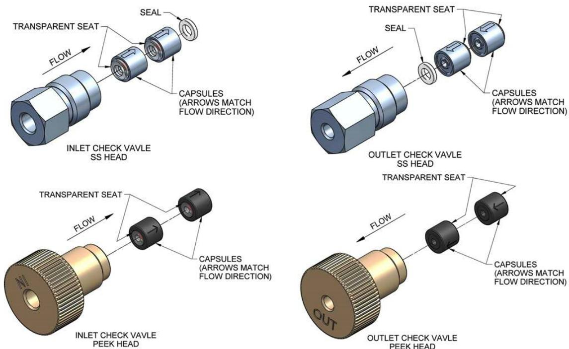
*Figure 10, Stainless Steel (SS) and PEEK Check Valves.*
