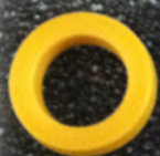
Figure 8, Example of polymer side vs. energizer side of seal.
