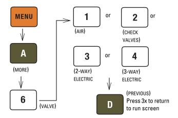
Figure 5-4 Keystrokes to specify valve type
