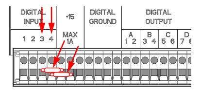
Figure 3-11 External resistor locations
