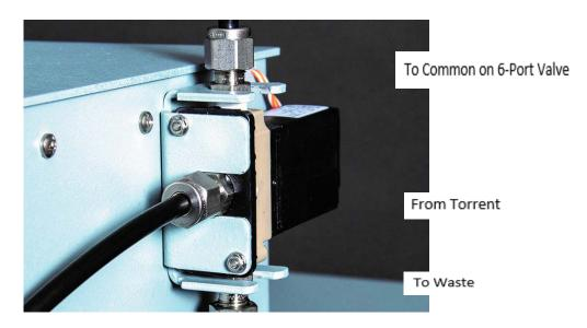
Figure 2-24 Fractionation value: Diverter to waste value connections
