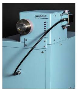
Figure 2-22 Fractionation Valve Plumbing to Torrent
