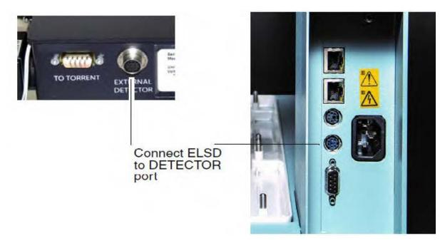
Figure 2-27 Detector port on fractionation valve (left) and Foxy R2 fraction collector (right)
