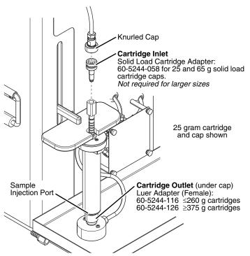
Figure 2-38 Changing cartridge inlet and outlet adapters
