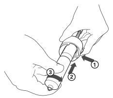
Figure 4-3 Align and push cartridge into the cap, and then rotate the cartridge to secure it.
