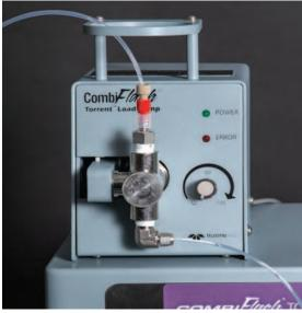
Figure 2-18 Plumbing Sample Inlet to Sample Loading Pump
