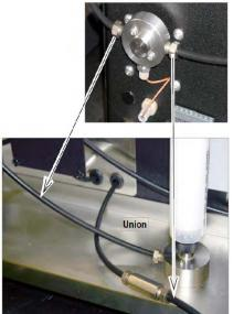
Figure 2-30 Tee fitting for Torrent ELSD
