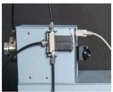
Figure 2-6 Electrical Connection between Fractionation Valve and Torrent
