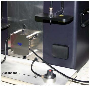
Figure 2-29 Replace the PEEK tee with the metal tee fitting
