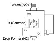
Figure 2-21 Foxy R2 high flow diverter value ports (front view)
