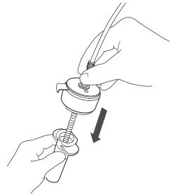
Figure 4-2 Insert the plunger to the bed
