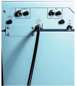
Figure 2-8 Solvent B Line connected to Solvent Selection Valve
