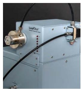
Figure 2-23 Fractionation Valve Diverter Valve to Fractionation Valve 6-Port Valve
