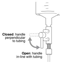
Figure 4-5 Liquid Injection Adapter
