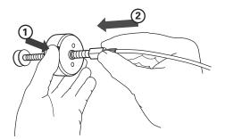
Figure 4-1 Press the lever and extend the plunger
