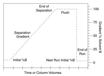
Figure 6-1 Default post-separation column and flow cell flush
