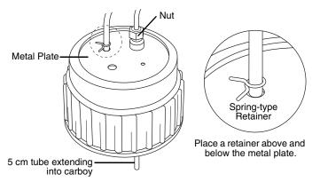
Figure 2-15 Optional Waste Cap (83B cap shown)
