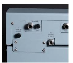
Figure 2-1 Solvent Select Valve mounted on Torrent
