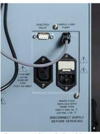
Figure 2-4 Sample Load Pump power supply connection on back of Torrent.
