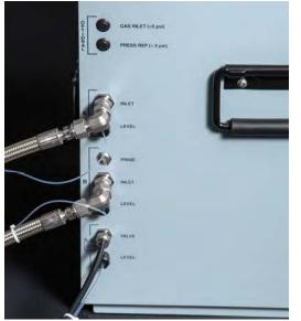
Figure 2-14 Waste Line connected to the Torrent
