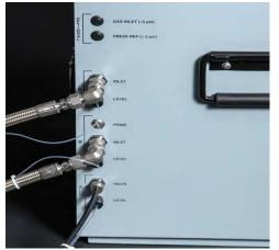
Figure 2-11 Solvent A line connected to the Torrent
