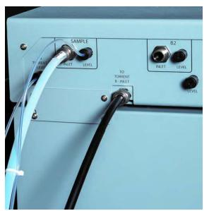
Figure 2-12 Sample Inlet Line connected to Solvent Selection Valve
