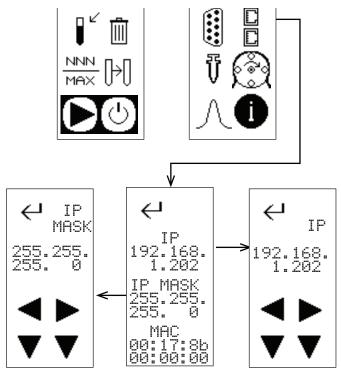
Figure 2-31 TCP/IP Settings for Foxy R2 Fraction Collector
