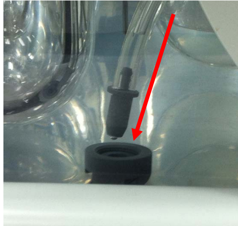
Fig. C-9 Insert the tubing from the syringe into the fitting
