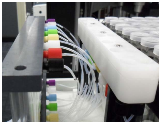
Fig. C-11 Waste Lines Attached to Retrieval Reservoir
