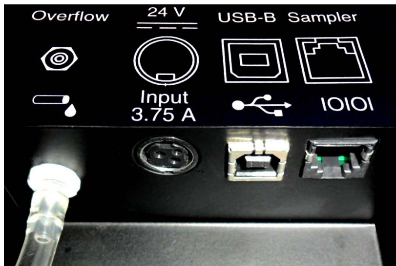
Fig. C-2 Photo of Vision AutoFill Back Panel and Ports
