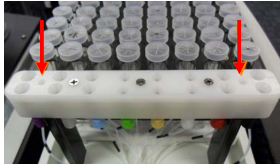
Fig. C-7 Home Port Screw Removal
