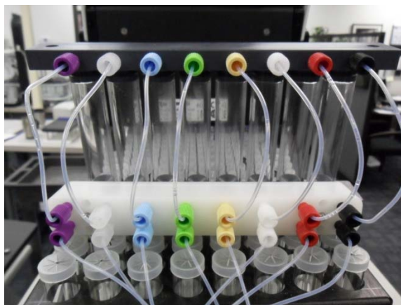
Fig. C-9 Connect Retrieval Reservoir Lines to the Home Port
