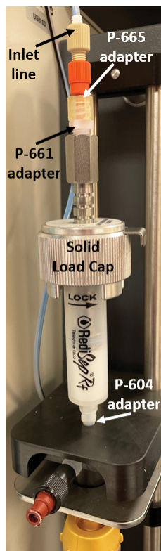
Figure 3. RediSep Solid Load Cartridge setup on a Büchi system.
