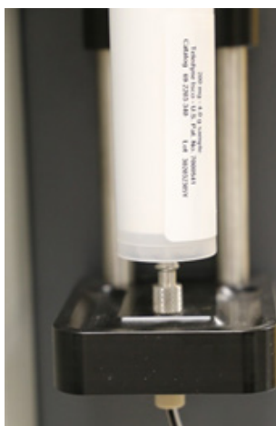
RediSep column installed on a system with an injection port shuttle
