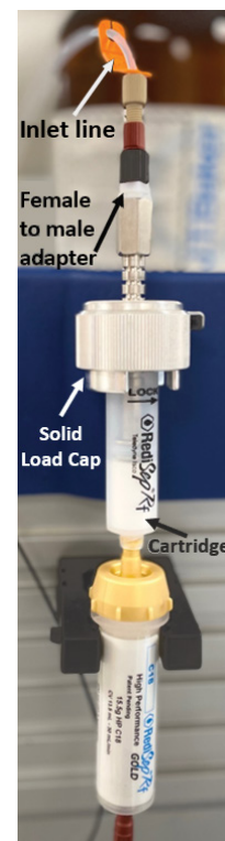
RediSep Solid Load Cartridge setup on system with tubing connections.
