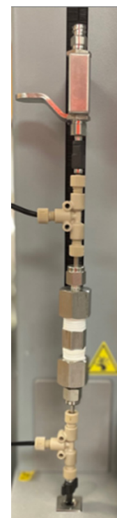
Large column attached connected to a column shuttle on a CombiFlash NextGen 300+
