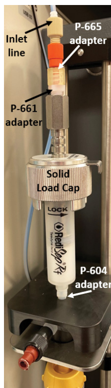
RediSep Solid Load Cartridge setup on system with a column shuttle
