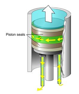
Figure 1: Illustration of wash gland operation
