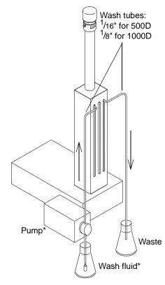
Figure 2: Wash fluid connections \*user-supplied
