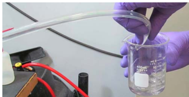
Figure 3: Draining the acetone into a 100 ml beaker
