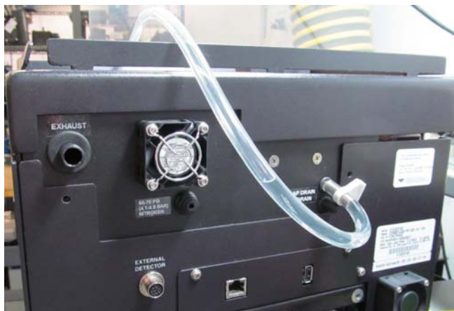
Figure 4: P-trap pump drain line draped over the unit
