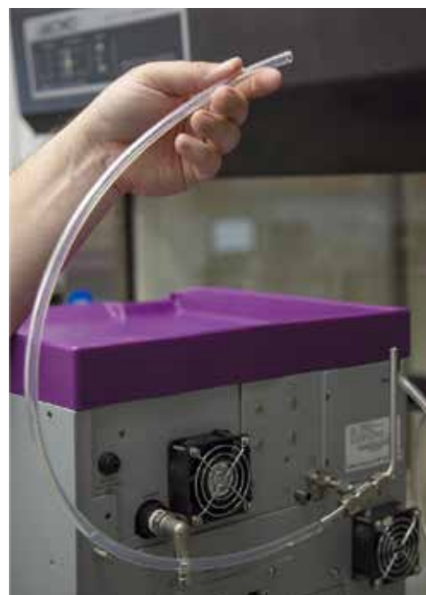
Figure 2: Filling the P-trap drain. Keep liquid level lower than the top of the system
