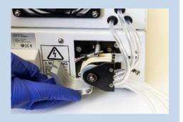
3. PEEK Sample Inlet Tubing Replacement. The sample inlet tubing assembly (made of PEEK) is used to deliver liquid sample to the U5000AT+ transducer which then converts the liquid sample into an aerosol. The end of the tubing may become worn with use and need replacement. Part number SP5150B contains one spare length of PEEK sample inlet tubing.
