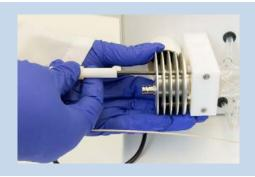
2. Drain Pump Tubing Replacement. The U5000AT+ is equipped with one 3-channel drain pump on the back panel of the unit to remove excess sample liquid and condensate. The drain pump tubing (light yellow color) has an expected lifetime of up to 6 months. Part number SP5366 contains (3) pre-cut spare drain pump tubing and (2) additional connectors.
