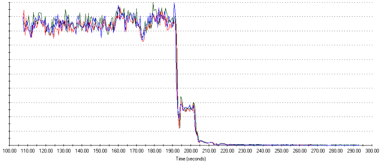
Figure 8 – Washout profile of 10 ppb tuning solution using the ASXPRESS PLUS system configured with an oils switching valve and a 1.02 ml aqueous sample loop using a segmented carrier stream pumped at \sim 300 \mu\text{l min}^{-1}
