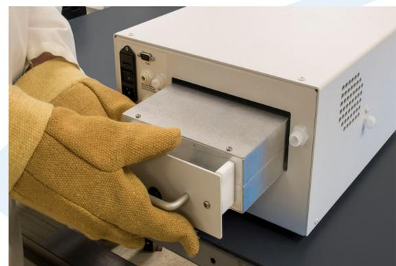
Figure 2. Removable Membrane Oven Module
