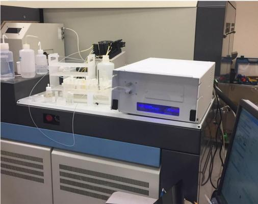
Fig 1. Thermo Fisher Neptune MC-ICP-MS w. Aridus3
