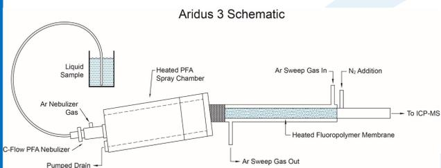
Figure 3. Aridus3 Schematic w. Gas Flows
