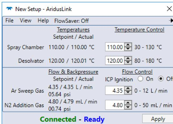
Figure 4. Aridus3 Software Control Screen of System Temperatures & Gas Flows
