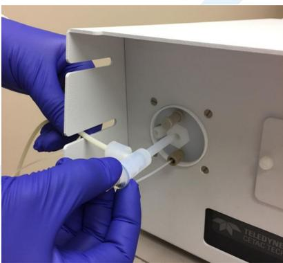
Fig 2. CFlow-100 PFA Nebulizer w. Aridus3 PFA Spray Chamber
