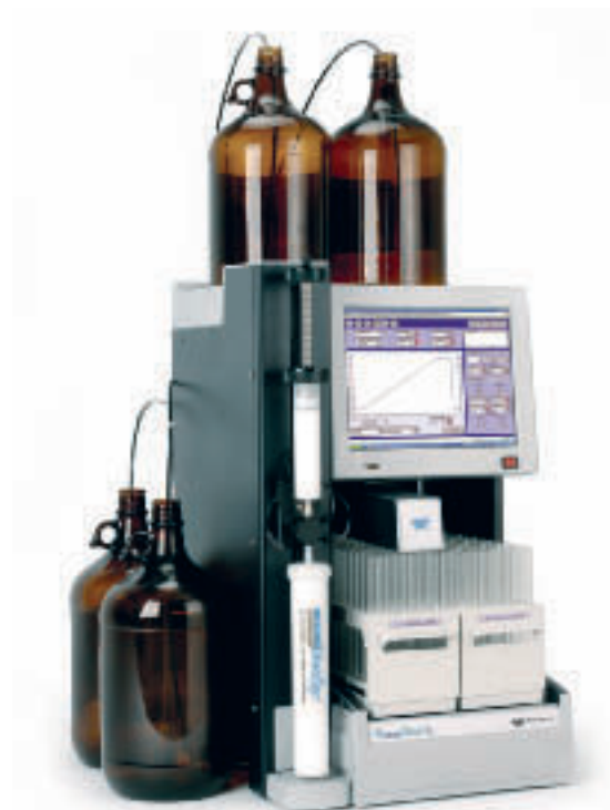
Figure 2. Teledyne Isco's CombiFlash Rf automated Flash chromatography system
