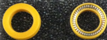
Figure 12, Example of polymer side vs. energizer side of seal. Note stainless steel energizer shown. Seal could have fluoropolymer o-ring energizer instead (black o-ring).
