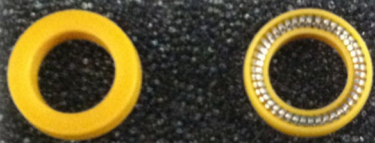
Figure 9, Example of polymer side vs. energizer side of seal. Note stainless steel energizer shown. Seal could have fluoropolymer o-ring energizer instead (black o-ring).
