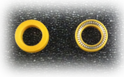
Figure 4-2, Example of polymer side vs. energizer side of seal. Note stainless steel energizer shown. Seal could have fluoropolymer o-ring energizer instead (black o-ring).
