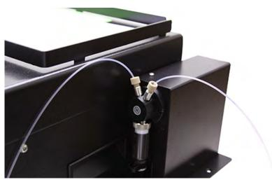
Figure 4-9 Waste line connected to the right AutoInjector Module port
