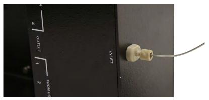
Figure 2-11 Column Selector Module inlet port
