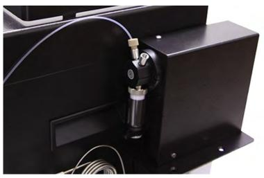
Figure 2-21 Connection of the waste tubing from the EZ Prep inject valve to the left  $AutoInjector\ Module\ port$
