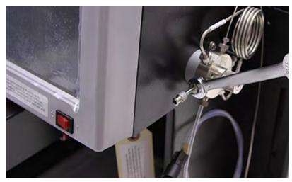
Figure 4-2 Removing the Luer fitting from the EZ Prep inject valve
