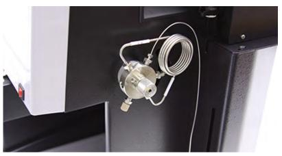
Figure 4-5 Waste tubing fitting attached to the EZ Prep inject valve
