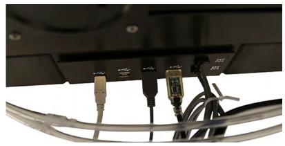
Figure~3-11 Auto Sampler~Module~USB-A~connection~(center)
