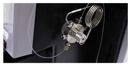
Figure 3-25 Sample probe tube fitting with the plastic fitting removed
