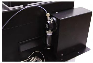
Figure 4-8 Connection of the waste tubing from the EZ Prep inject valve to the left AutoInjector Module port
