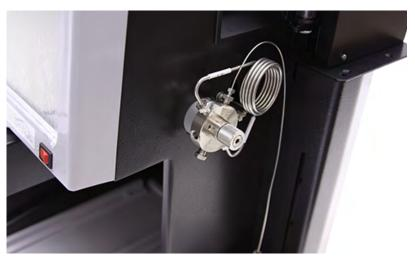
Figure 4-6 Waste fitting with the plastic fitting removed
