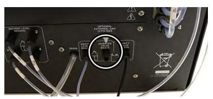
Figure 3-21 Diverter Valve Waste port with no connection
