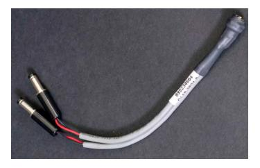
Figure 2-27 Y-Type power supply
