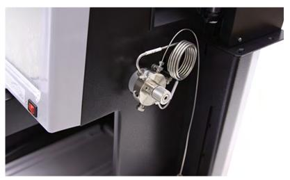
Figure 2-19 Waste fitting with the plastic fitting removed
