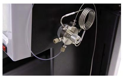
Figure 2-24 Sample tube fitting attached to the EZ Prep inject valve
