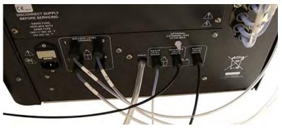
Figure 3-22 Diverter Valve Waste port with AutoSampler Module tubing connection
