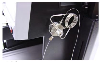
Figure 2-20 Waste fitting with tubing attached
