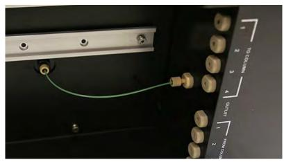
Figure 2-13 Connected Column Selector Module outlet port tubing
