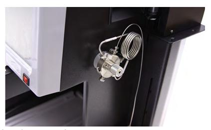
Figure 3-29 Waste fitting with the plastic fitting removed
