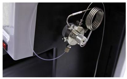
Figure 2-25 Sample tube fitting with the plastic fitting removed
