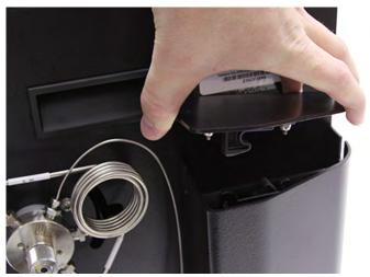
Figure 4-1 Removing the top cover of the EZ Prep column mount
