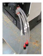
Figure 3-6 AutoSampler Module peristaltic pump with tubing correctly attached
