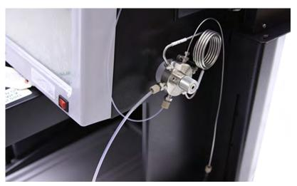
Figure 4-13 Sample tube fitting with sample tubing attached
