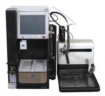
Figure 3-35 EZ Prep system with the AutoSampler
