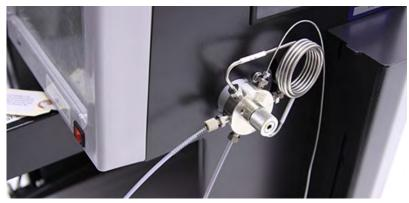
Figure 3-26 Sample probe tube fitting with sample probe tubing attached
