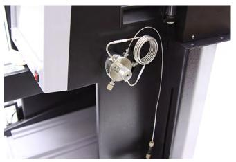
Figure 2-18 Waste tubing fitting attached to the EZ Prep inject valve
