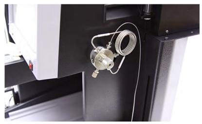
Figure 3-28 Waste tubing fitting attached to the EZ Prep inject valve
