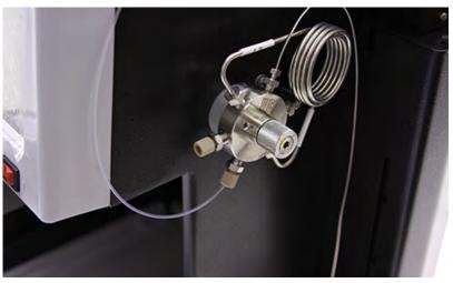
Figure 4-11 Sample tube fitting attached to the EZ Prep inject valve
