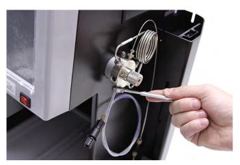
Figure 2-17 Removing the waste line from the EZ Prep inject valve
