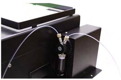
Figure 2-22 Waste line connected to the right AutoInjector Module port
