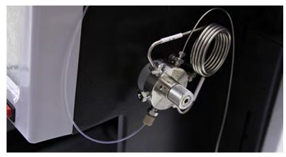
Figure 4-12 Sample probe tube fitting with the plastic fitting removed
