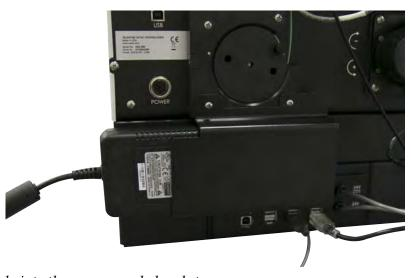
Figure 3-16 Inserting the power supply into the power supply bracket
