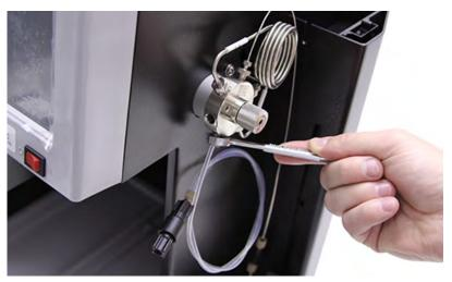
Figure 4-3 Removing the waste line from the EZ Prep inject valve
