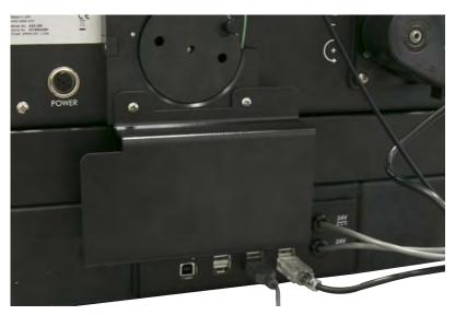
Figure 3-15 Power supply bracket secured to the AutoSampler Module
