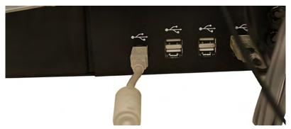
Figure 3-20 AutoSampler Module USB-B connection
