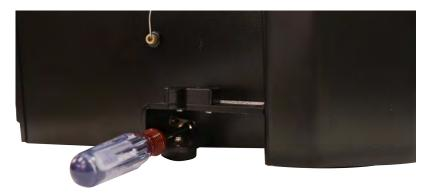
Figure 2-2 Removing the bottom section housing nut
