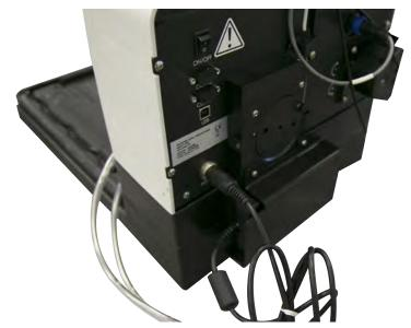
Figure 3-17 AutoSampler Module with power connection made
