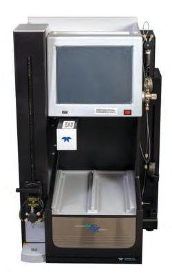
Figure 4-14 AutoInjector mounted on the EZ Prep
