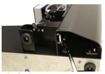
Figure 2-3 Removing the EZ Prep housing column inner nut
