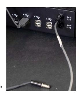
Figure 3-1824 V Power supply cane and the port on the back of the EZ Prep
