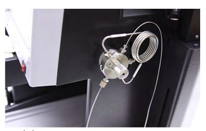
Figure 4-7 Waste fitting with tubing attached
