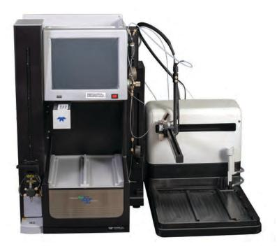
$Figure~4-15\,Auto Sampler~installed~with~an~Auto Injector\\mounted~on~the~EZ~Prep$
