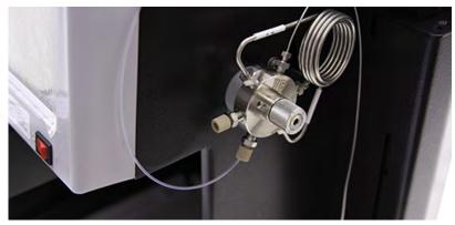
Figure 3-24 Sample probe tube fitting connected to the EZ Prep inject valve
