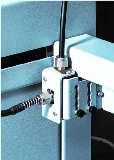
*Figure 2-20 Plumbing at the Foxy R2 Diverter valve*
