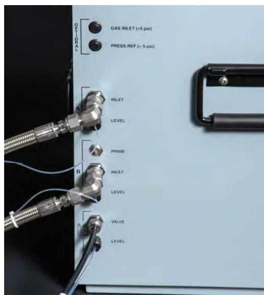
Figure 2-14 Waste Line connected to the Torrent
