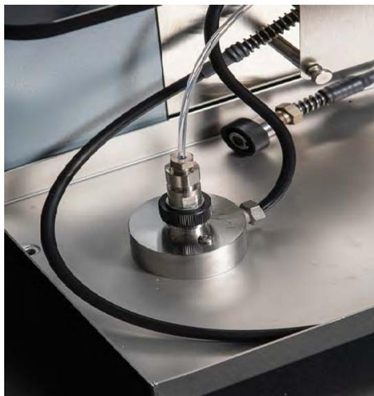
*Figure 2-16 Sample Load Pump connected to the Torrent Sample Injection Port.*
