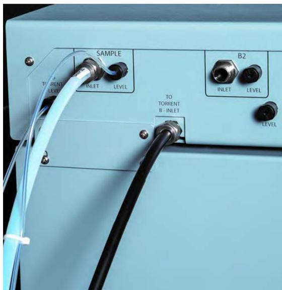
Figure 2-12 Sample Inlet Line connected to Solvent Selection Valve
