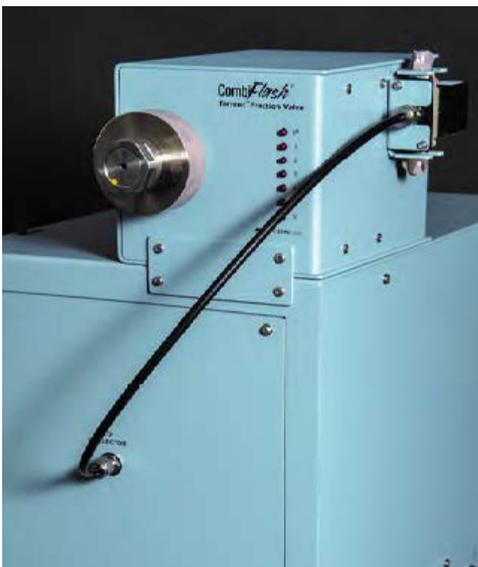
Figure 2-22 Fractionation Valve Plumbing to Torrent
