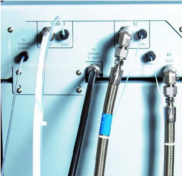
Figure 2-13 Solvent B1 and B2 supply lines connected to Solvent Selection Valve
