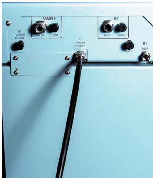
*Figure 2-8 Solvent B Line connected to Solvent Selection Valve*
