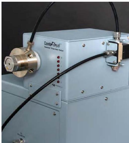
Figure 2-23 Fractionation Valve Diverter Valve to Fractionation Valve 6-Port Valve
