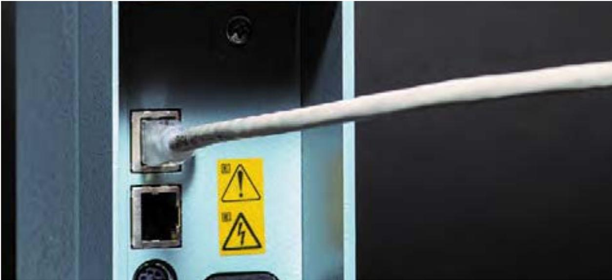
Figure 2-7 Connection on back of Foxy R2 Fraction Collector to the Torrent
