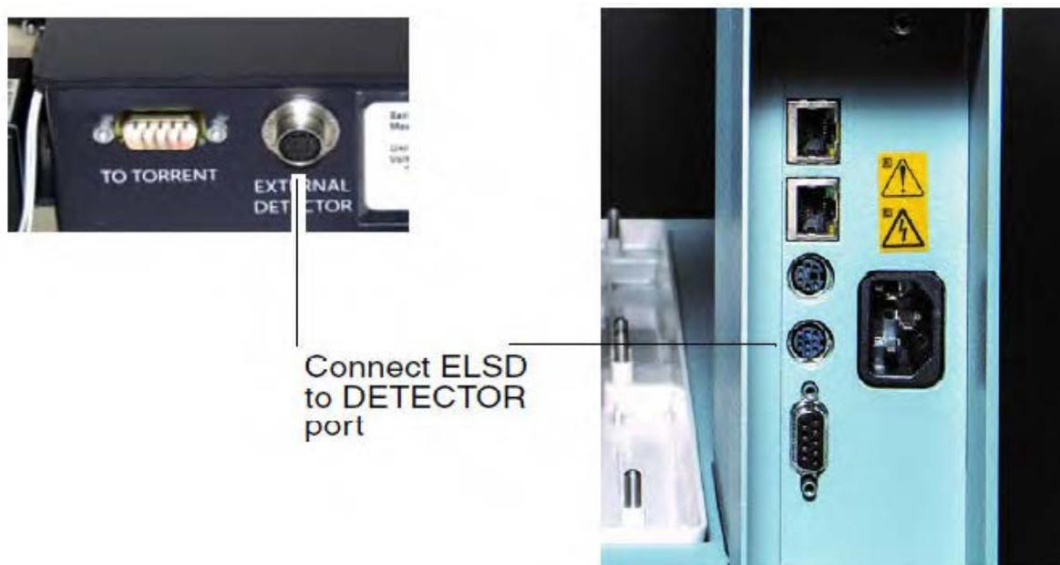
Figure 2-27 Detector port on fractionation valve (left) and Foxy R2 fraction collector (right)
