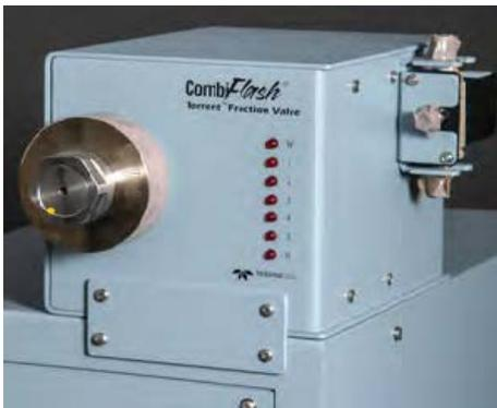
*Figure 2-3 Fractionation valve after mounting*
