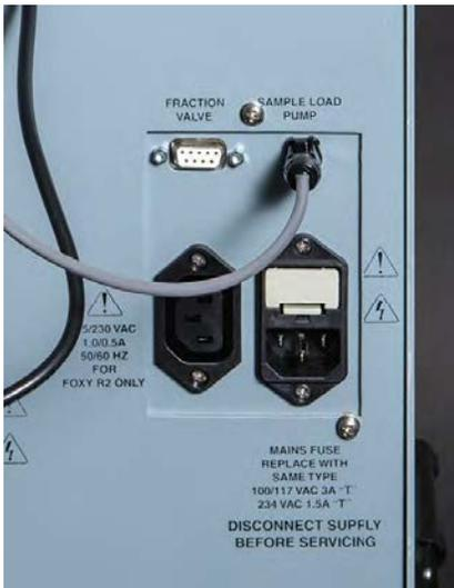
Figure 2-4 Sample Load Pump power supply connection on back of Torrent.
