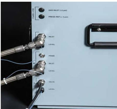
Figure 2-11 Solvent A line connected to the Torrent
