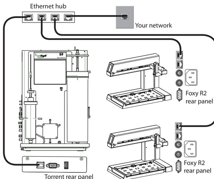
Figure 2-17 Network configurations: Example 3
