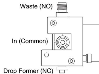
Figure 2-4 Foxy R2 high flow diverter valve ports (front view)
