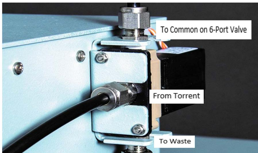
Figure 2-5 Fractionation valve: Diverter to waste valve connections
