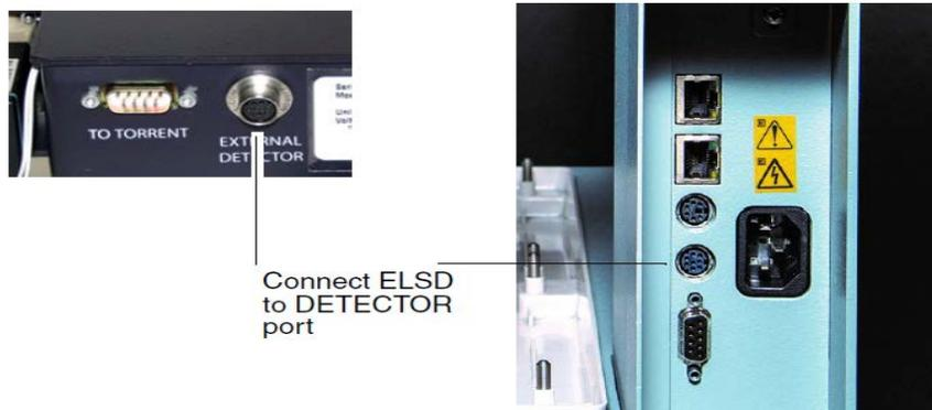
Figure 2-7 Detector port on fractionation valve (left) and Foxy R2 fraction collector (right)
