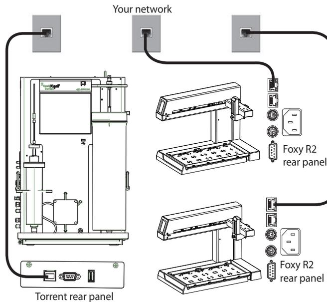
Figure 2-16 Network configurations: Example 2
