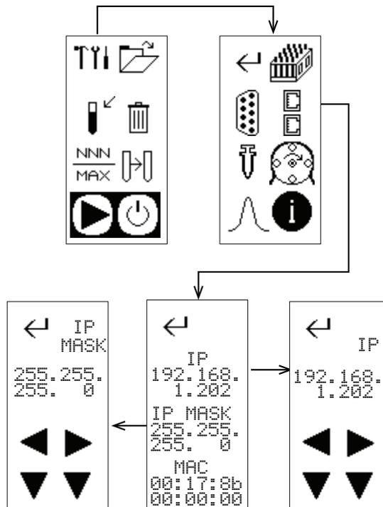
Figure 2-12 TCP/IP Settings for Foxy R2 Fraction Collector
