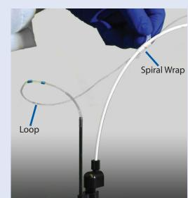
Connect the Sample Tubing to the Analytical Instrument
