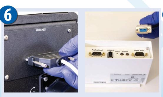
Connect ASX 560 I/O Board to ÄKTA I/O Box
