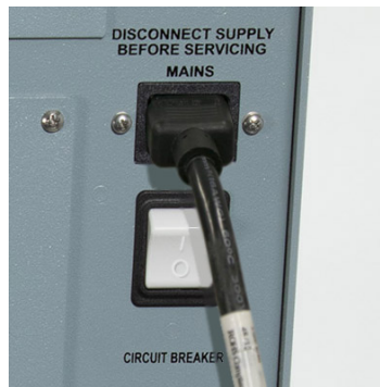
Figure 1-2 Location of the control box power cord and breaker
