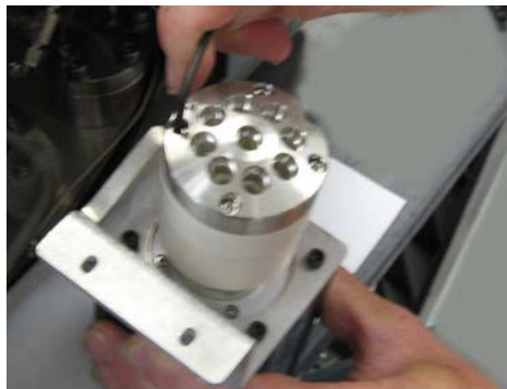
Figure 5-14 Loosening of the fractionation valve stator
