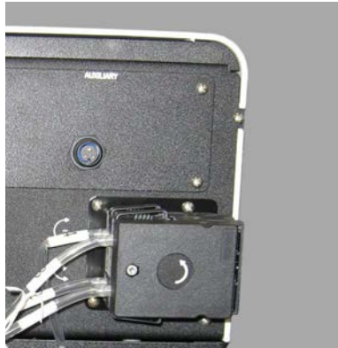
Figure 5-20 The peristaltic pump at the back of the AutoSampler
