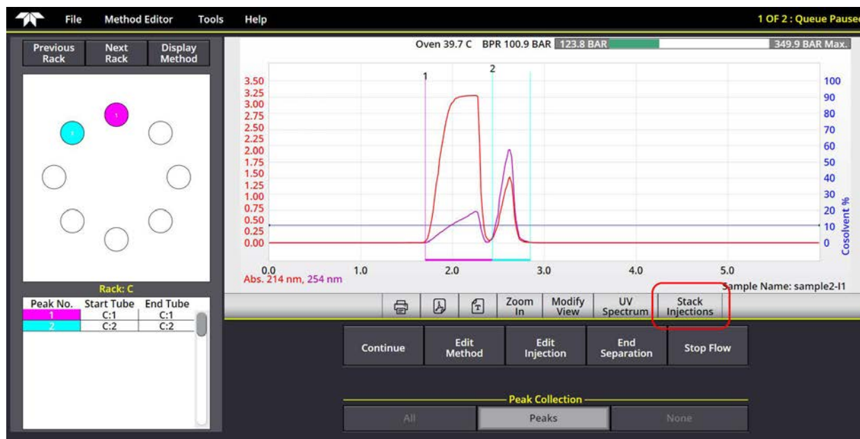
Figure 3-16 Higher sample loading, ready for stacked injections
