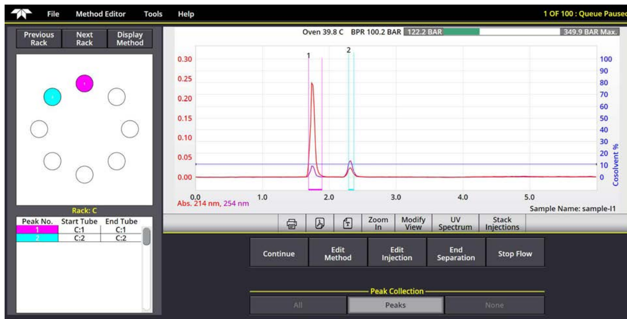
Figure 3-14 Chromatogram showing High Resolution at the end of a run
