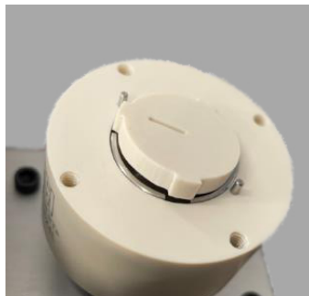
Figure 5-16 Removal of the fractionation valve rotor
