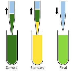
**Serial Dilution** – Programmable rinsing and mixing options make it easier than ever to do accurate and simple serial dilutions.
