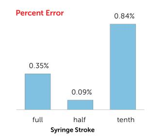
**Precision** – It is not enough to hit the target once; the SimPrep hits the target every time. Variations from sample to sample can lead to serious problems for any analysis. This is a particular challenge with hand pipetting, and one that is removed by the automation provided with the SimPrep. In the figure at right you can see the data summarized from three sets of 10 replicates at different dilution levels.
