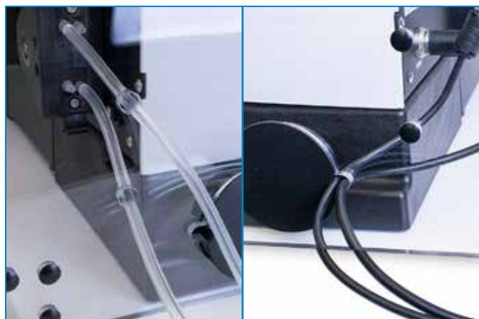
Multiple egress ports provide convenient access to tubing and power cords for any laboratory and ICP setup.
