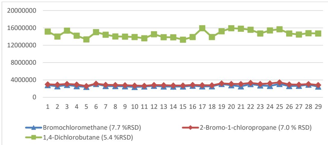
**Figure 4** Graph of the Calculated Surrogate Standards 30 ppb Concentration and their Respective %RSD from 29 Samples During Approximately 10 Hours of Testing.
