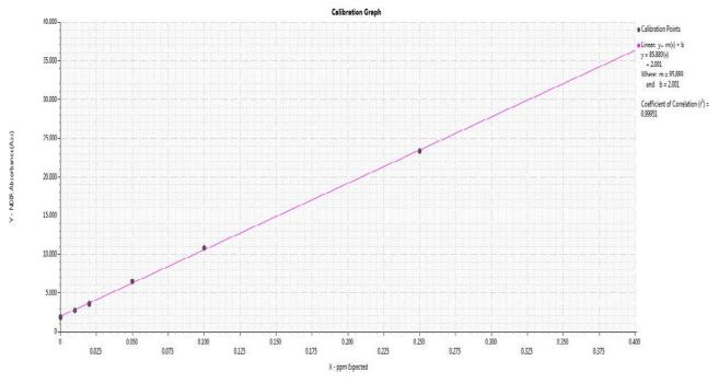
Figure 3: Calibration curve for the low level TOC analysis
