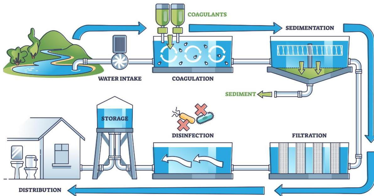
Figure 1 Typical Water Treatment Process for Drinking Water
