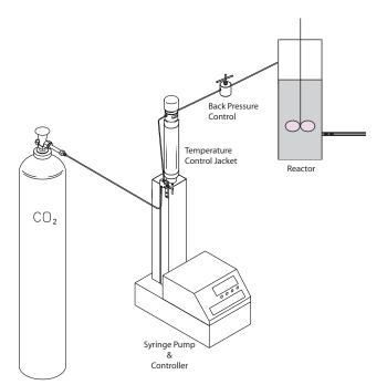
Figure 3: Configuration for stable mass delivery rate of  $CO_2$  to reactor
