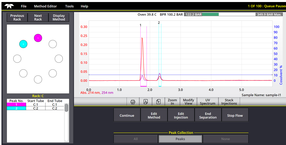
Figure 2. End of run — there is a lot of resolution, so the injection volume will be increased.
