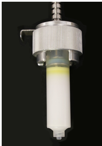
Figure 4: Yellow material on the silica is irreversibly bound material which otherwise would be adsorbed on the reverse phase column.
