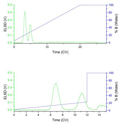
**Figure 3.** Fructose and sucrose purified using an acetone/water gradient. A 15.5 g RediSep Gold amine was used for the scouting run.
