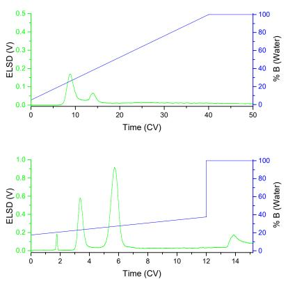
**Figure 1.** Ribose and glucose run in a scouting method on a 5.5 g RediSep Gold Amine column (top) and focused to a 50 g RediSep Gold amine column. The total sample load was 50 mg each of ribose and glucose. The small peak at ~1.8 column volumes in the focused gradient is DMSO.
