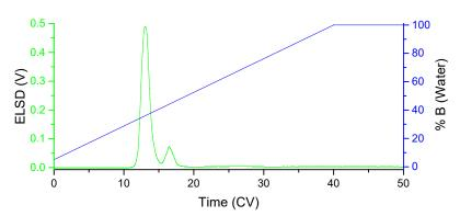
**Figure 2.** Purification of impure fructose from sucrose using RediSep Gold Amine columns and an acetonitrile/water gradient.
