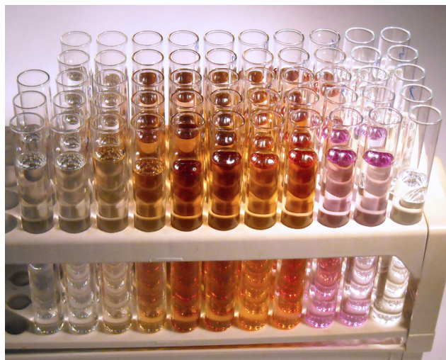
Figure 2: Fractions on right exhibited the characteristic purple color of purified C 60 fullerene
