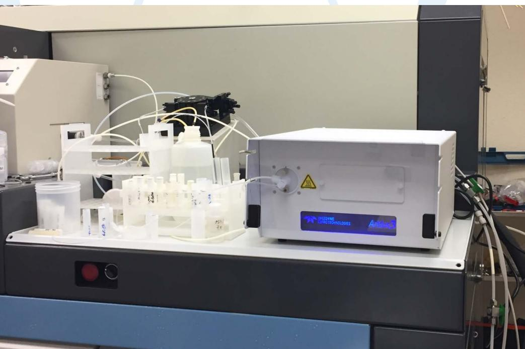
Figure 3. ThermoFisher Neptune MC-ICP-MS & **Teledyne CETAC Aridus 3 Desolvating Nebulizer**
