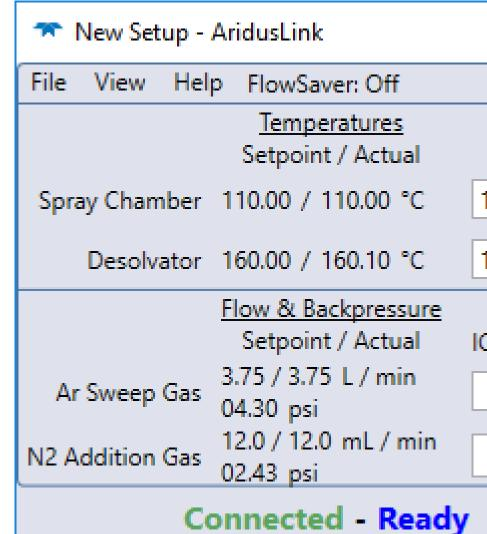
Figure 4. AridusLink Software Control Screen
