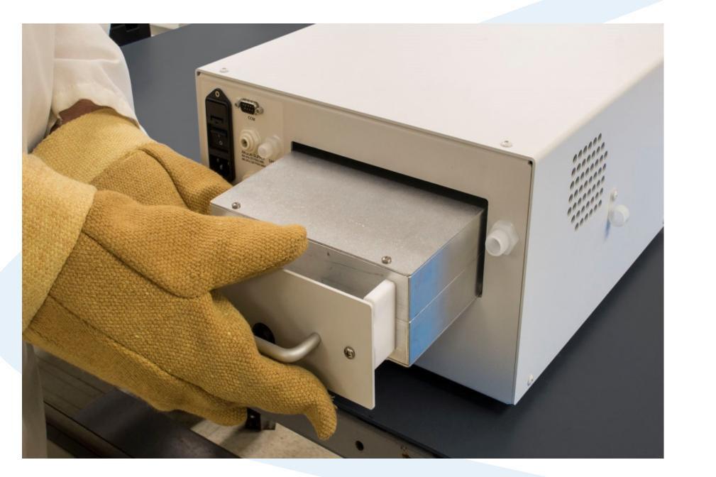
Figure 2. Removable Membrane Oven Module
