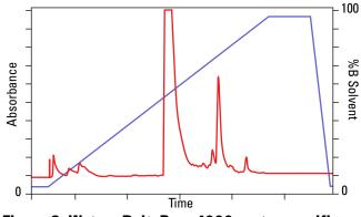
Figure 3: Waters DeltaPrep 4000 system purification of 10 mg sample of Compound A using a Vydac 10x250 mm column, 5µ particle size
