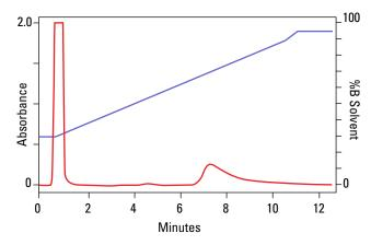
Figure 6: Protected Aminoglycoside purified on a standard C18 Flash column on a Combi*Flash* Companion system
