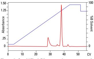
Figure 2: Combi*Flash* Rf system chromatogram of 46 mg purification of Compound A on a 15.5g Redi*Sep* Rf Gold C18 column
