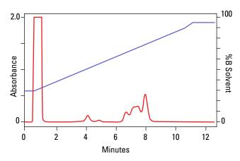
**Figure 7: Protected Aminoglycoside purified on a Redi***Sep* **Rf Gold C18 Flash column** on a Combi*Flash* Companion system
