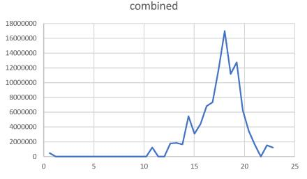
Figure 4—Combined mass traces to identify AS-48 elution.
