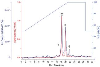
Figure 4: Final capsaicin purification on prep HPLC column
