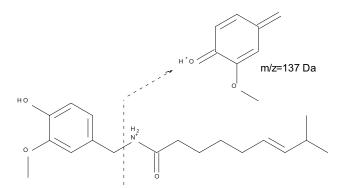
Figure 2: Schematic representation of the daughter ion produced from capsaicin at m/z = 137 Da
