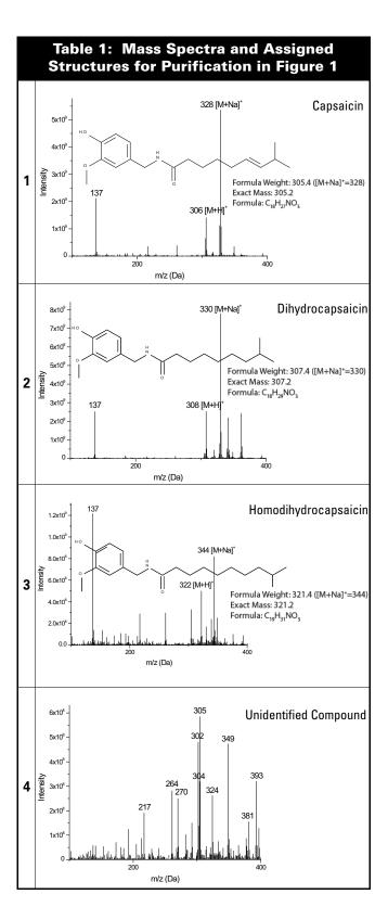
A fragment common to the capsaicin compounds is the peak at m/z=137 created from the phenolic portion of the molecule (Figure 2)<sup>5</sup>. This fragment allows easy identification of those peaks which are capsaicinoids from those peaks not containing this compound family. For example, peak 4 in Figure 1 and Table 1 does not exhibit this fragment and is therefore presumed not to be a capsaicinoid.
