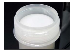
Figure 3: Reservoir Column showing equilibration solvent which requires removal before loading sample
