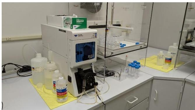
**Figure 4** QuickTrace® M-7600 CVAA Peristaltic Pump W/Smaller ID tubing
