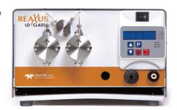
Chromatography (HPLC). Standard fluid path materials are Stainless Steel and PEEK. Other available features include Hastelloy fluid path with jacketed pump heads for temperature controlled applications. With 12 mL/min, 36 mL/min, and 100 mL/min versions, reaching pressures up to 6,000 psi, these pumps will meet the performance requirements of demanding HPLC needs.
