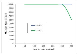
*HF Series pumps have an open voltage input of 90–260 Volts AC. The chart above shows the capabilities at 110 Volts and 220 Volts.*
