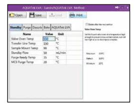
Method Development Screen - The Lumin TekLink™ software comes pre-installed with methods for most applications. You can select one of these methods or if your application calls for a unique requirement, a customized method can be created to meet your analytical requirements for sample processing.
