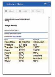
**Instrument Status Screen** - The Instrument Status screen provides valuable information such as mode of operation and instrument conditions. During Leak Check, it displays the region of the system that is being checked and the time remaining of the leak check.
